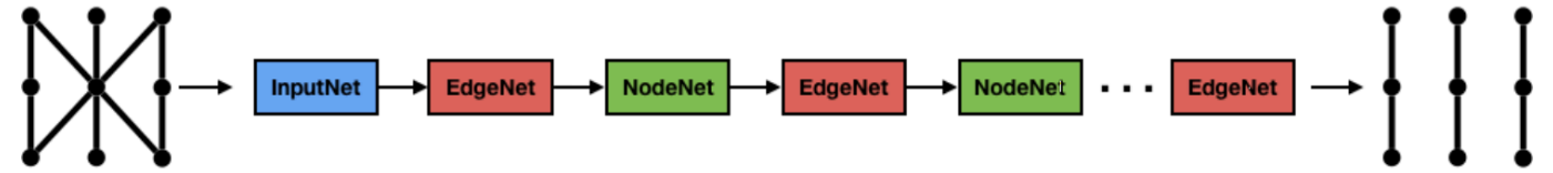
Figure 9. Diagram of the Graph Neural Network model which begins with an input transformation layer and has a number of recurrent iterations of alternating EdgeNetwork and NodeNetwork components. In this case, the final output layer is the EdgeNetwork, making this a segment classifier model.
