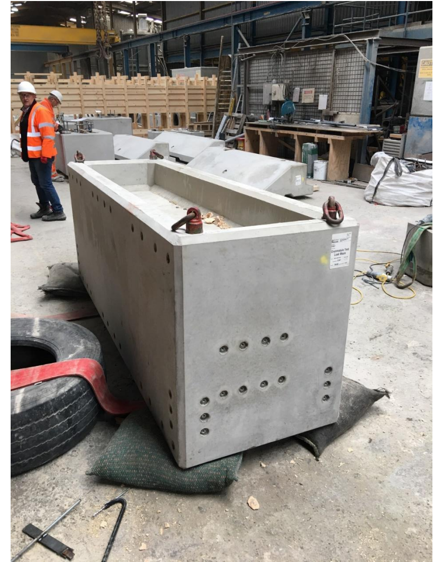
Test Block has been cast
