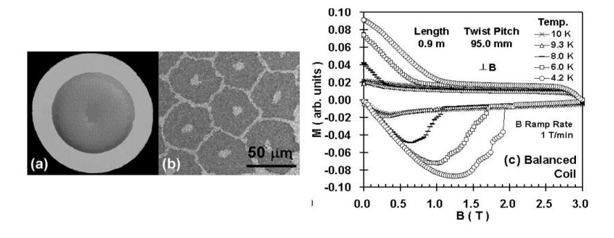
Magnetization curve of reacted Nb3AI strands, tested using a balanced coil magnetometer
