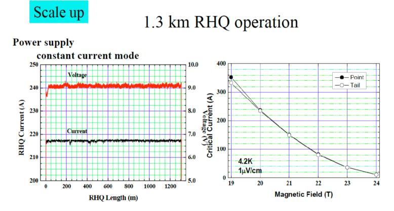
Small fluctuation of inter-electrode voltage and current over the whole length of RHQed wire **Little difference in**  $I_c$  between a head (point) and a tail of 1.3 km-length of wire
