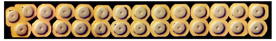
Size (rectangular): 14.2 mm x 1.8 mm Compaction Factor: 89.1 % Lay Angle: 15.0
