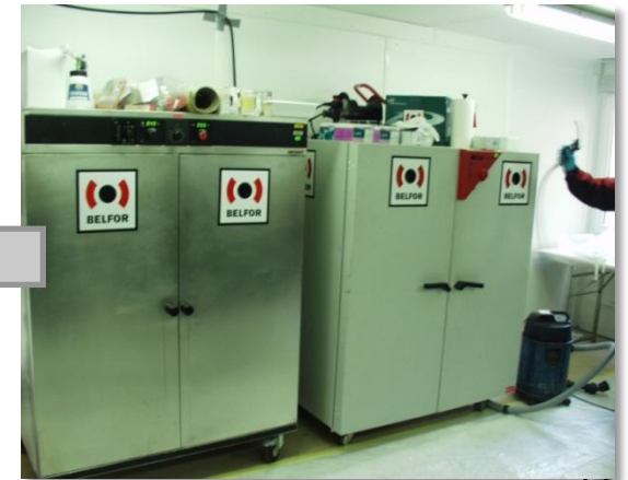
Ovens for drying after chemical cleaning
