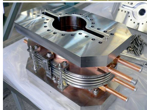
Antechamber being tested in KEKB
