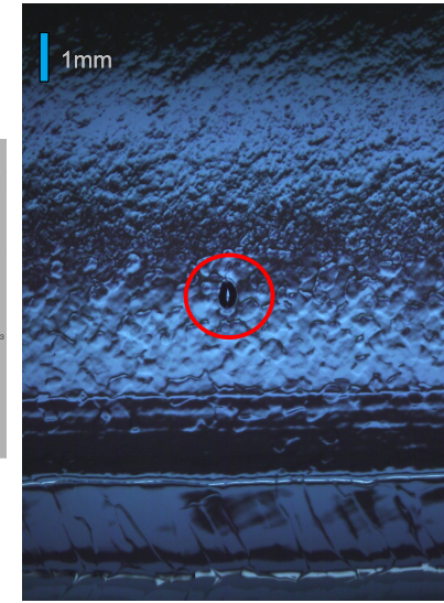
Correlations of Temperature Map and Optical Features on the Nb cavity inner surface
