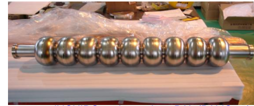
9-cell ICHIRO cavity made at PAL (PALIC #1)
