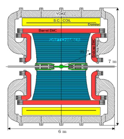
**Superconducting coil** *B* = 0.52 T
