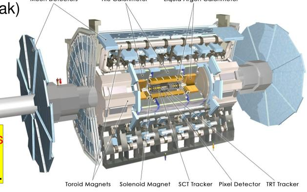
HAD calorimeter - 3 sections covering up to |η|≈5 Good containment, good resolution for jet measurement
