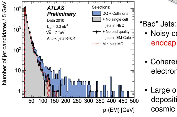
Noisy cells in the hadronic endcap calorimeter (HEC)
