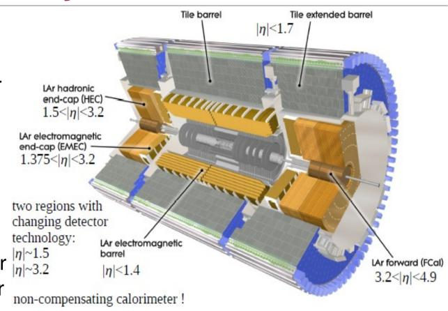
Forward calorimeter:  $3 < |\eta| < 4.9$ . First layer EM (Cu/LAr), the two remaining layers HAD.
