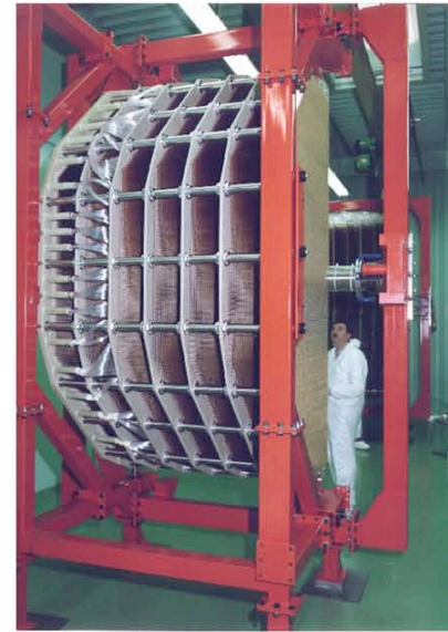
NA48 (CP violation in K^0 ) LKr calorimeter
