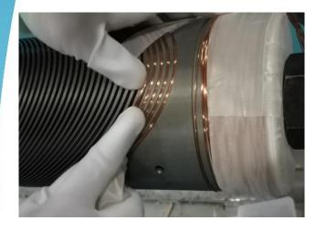
September 10, 2020 Winding of inner former completed
