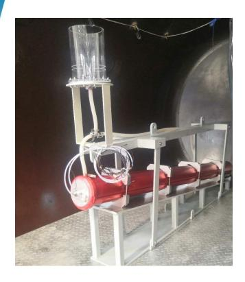
October 1, 2020 VPI tooling assembly and precuring completed. Moved to VPI furnace
