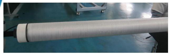
October 23, 2020 Inner coil winding of the 1st magnet V aperture Completed "dry winding"
