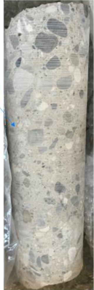
Slab core drilling in a maintenance pit
