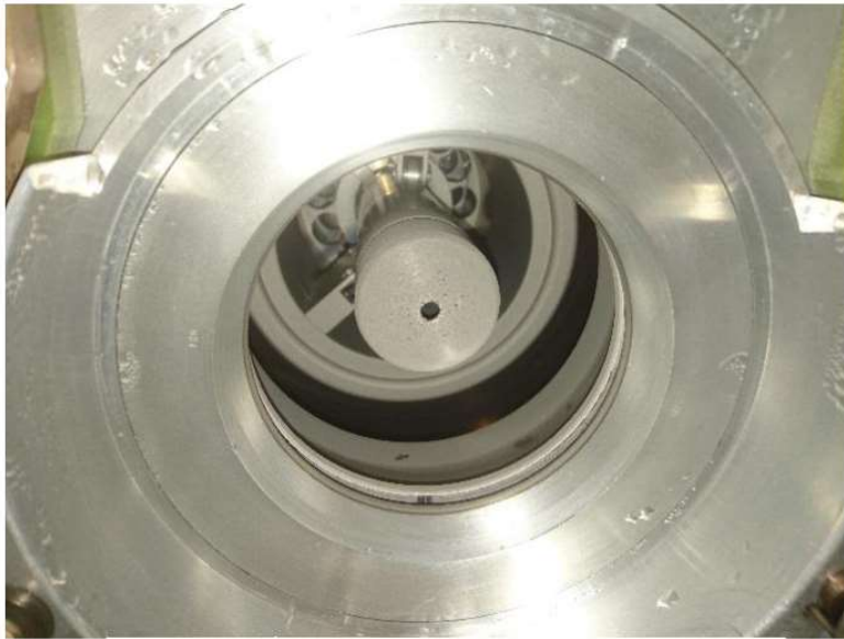
Figure.32: Extraction electrode coated with LBE
