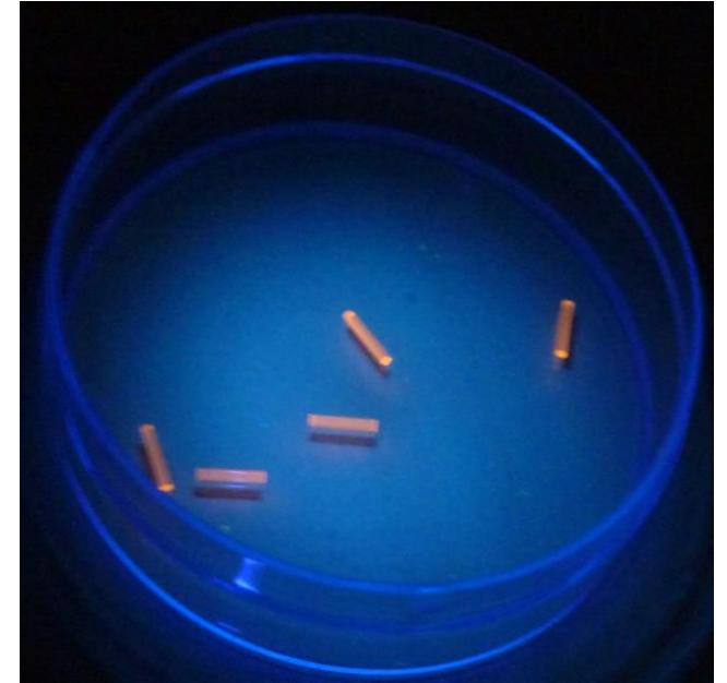
Irradiated RPL dosimeters when being illuminated with UV light
