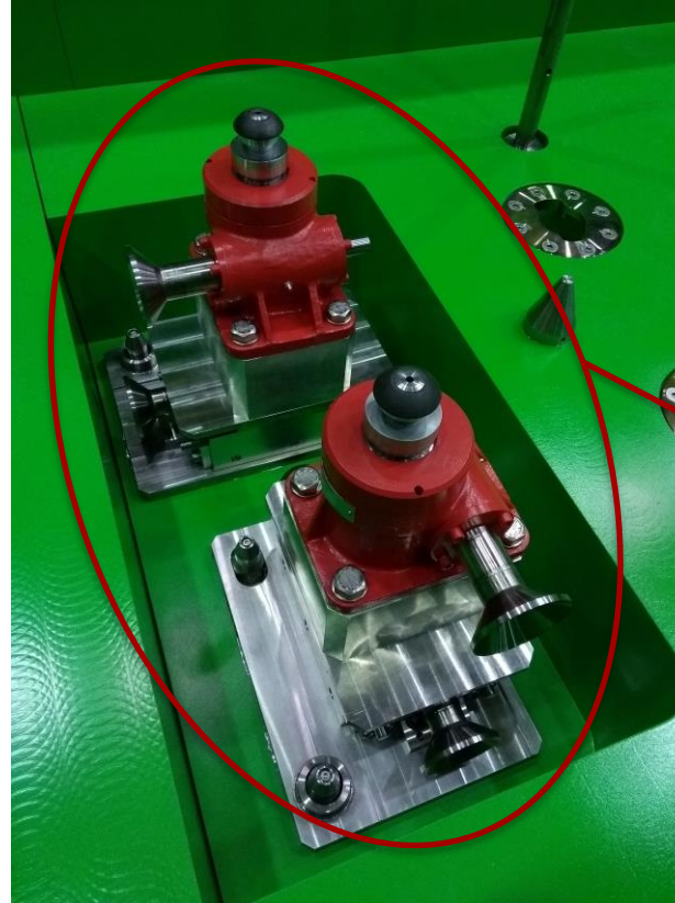
Support jacks inside shielding SY-STI, 2020.
