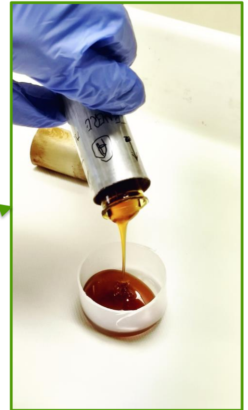
Aspect of MORESCO RP-42R after irradiation M.Ferrari, Ph.D. Thesis (2020); EDMS 2412825
