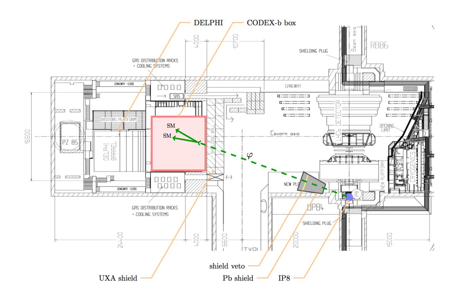
CODEX-b is a similar distance to the IP as LHCb's muon spectrometer From Run 3 onwards LHCb will operate a triggerless full detector readout @ 30 MHz Therefore go for the simplest solution: integrate CODEX-b "as another subdetector"
