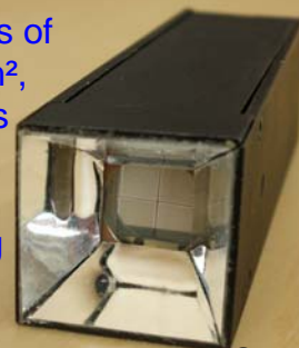
A 22mmx22mm SiPM based pixel for a telescope
