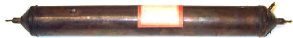
A Geiger-Müller counter built in 1939 and used in the 1947-1950 for cosmic ray studies in balloons and on board B29 aircraft by Robert Millikan et al.
