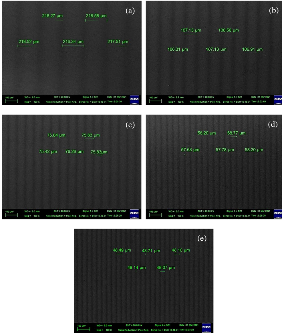
Figure 2. Image of reflective holographic gratings obtained by SEM, where (a) Sample 1, (b) Sample 2, (c) Sample 3, (d) Sample 4, and (e) Sample 5.
