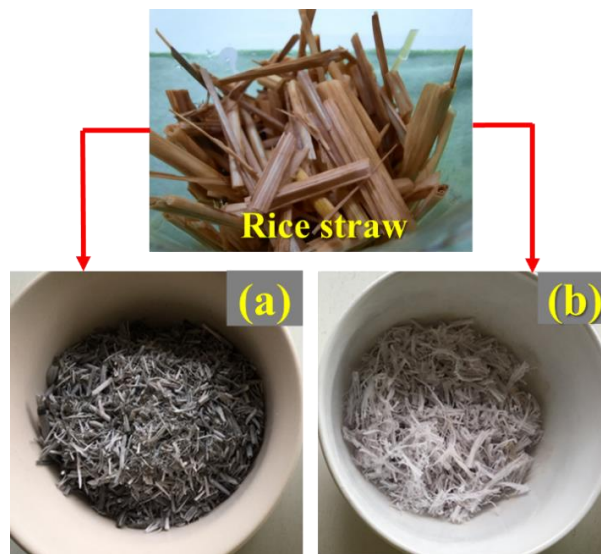
Figure 2. Color of rice straw ash from rice straw, (a) un-treated and (b) treated, by 0.1 M HCl.
