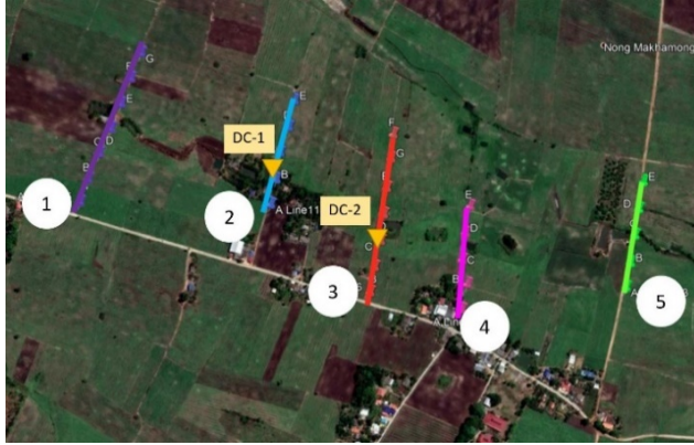
Figure 3. 2D-resistivity survey lines consist of 5 lines with total length of 1,415 m and locations of drilled wells (DC-1 and DC-2) on survey lines.
