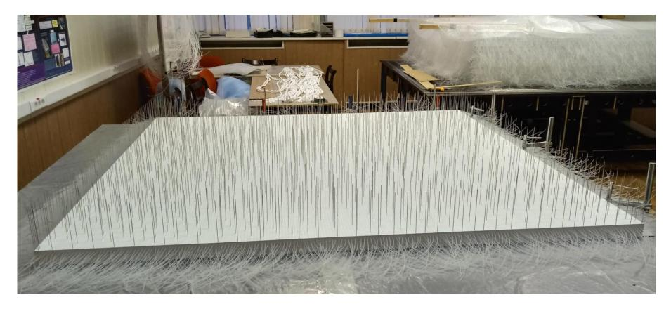
Two layers are merged simultaneously. Merging means the vertical alignment of holes. All 5 layers are aligned with 1.4 mm diameter needles.
