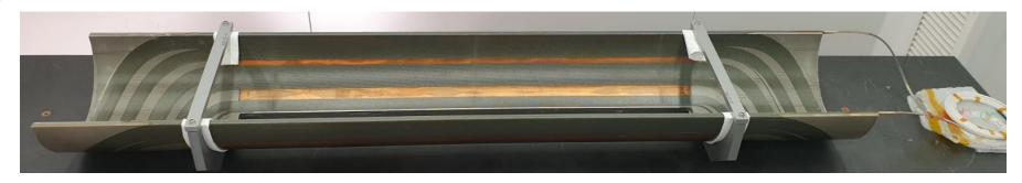
Winding of the second outer dipole coil outer layer in progress:
