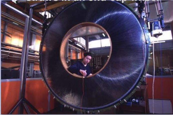
straws in an end-cap wheel
