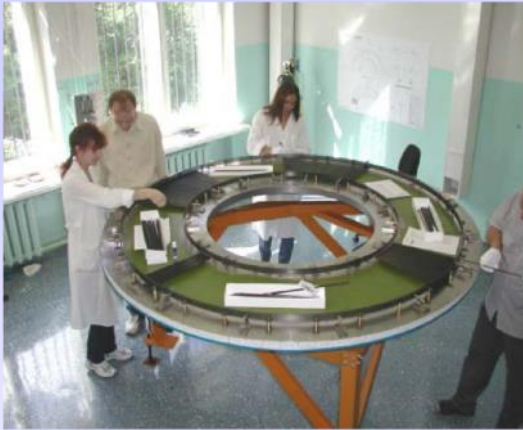
Installation of straws (tests leak tightness)
