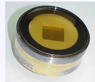
Sealed gaseous photodetector with bialkali PC. (Weizmann Inst., Israel)
