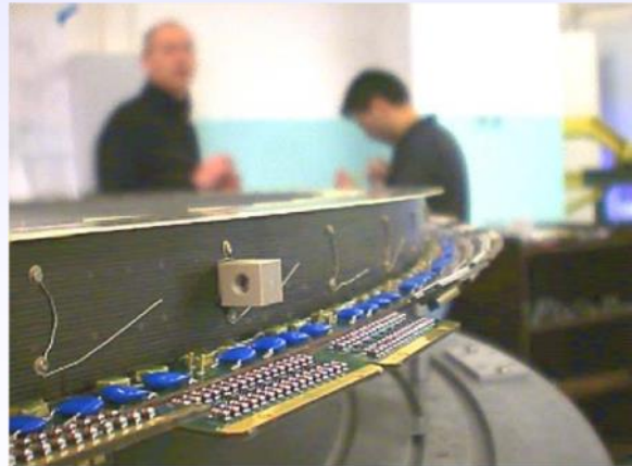
Sealing of wheel (tests leak tightness & HV)
