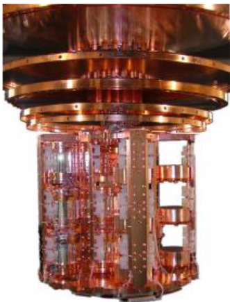
The CRESST Detector Modules are arranged in a support structure which can hold up to 33 crystals, corresponding to 10kg of detector material.
