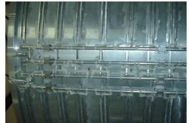
Thermal siphon cooling layout, pipework welded to the cylinder
