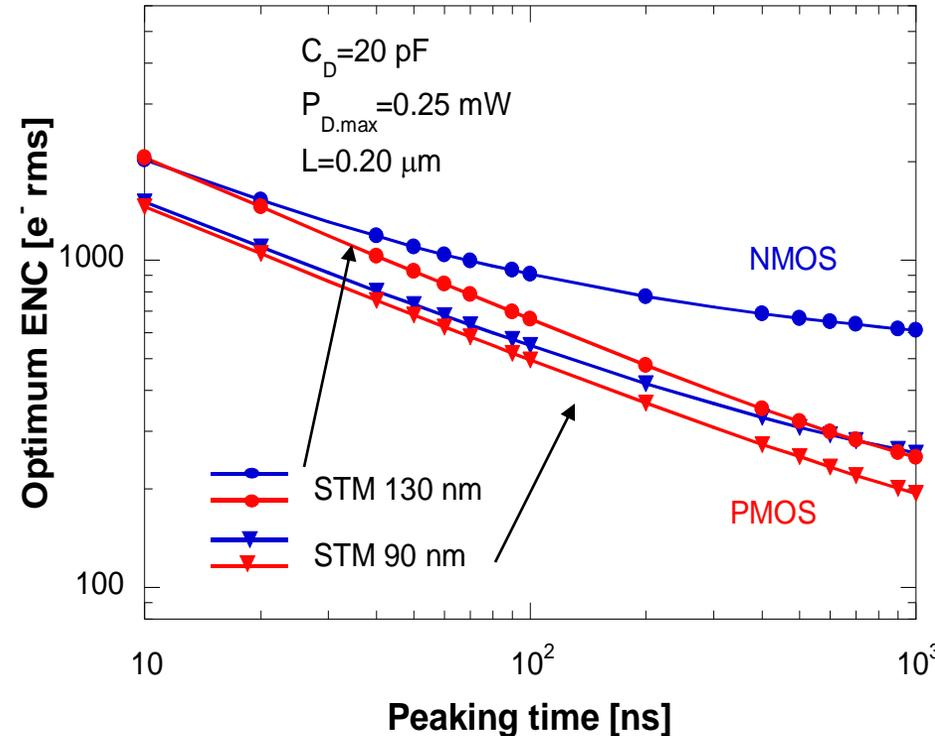
ENC was evaluated in the case of a second order, unipolar (RC<sup>2</sup>-CR) shaping processor
