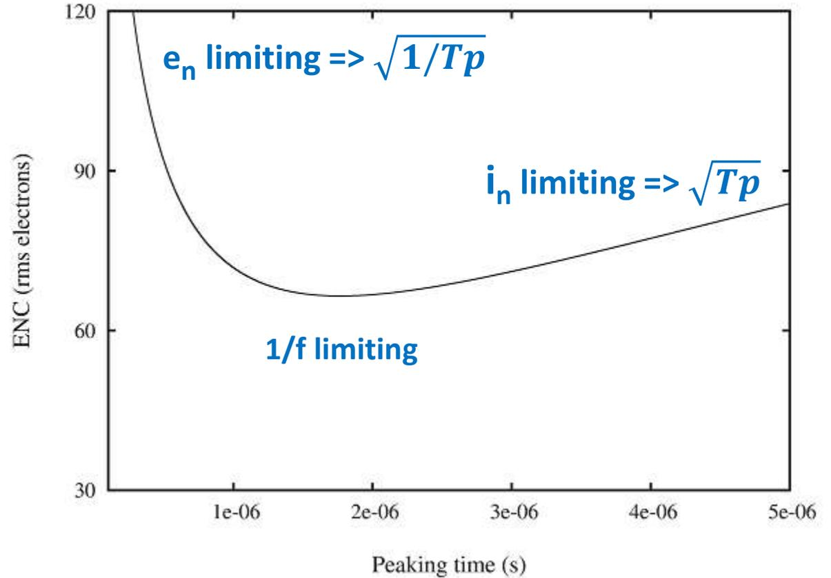
$$ENC^2 = (C_d + C_{in})^2 \left( A_w v_n^2 \frac{1}{T_p} + A_f K_f \right) + A_p i_n^2 T_p$$
