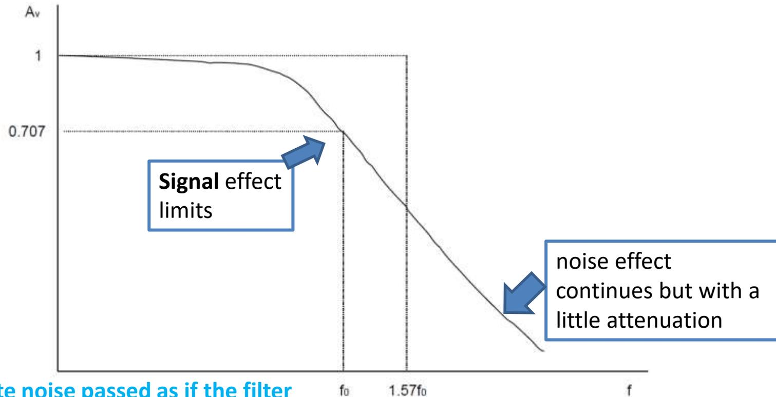
The white noise passed as if the filter were a brick wall type but with a cutoff freq 1.57 times larger
