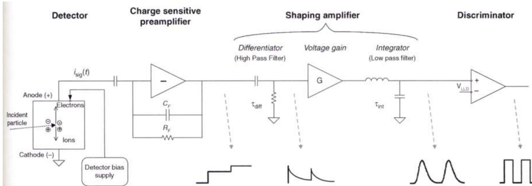
Schematic of simple signal processing electronics. This circuit is suitable for use, as shown, in many applications and is conceptually similar to more complex circuits. These elements are discussed in greater detail in Chapter 17. (Courtesy of R. Redus, Amptek, Inc.)
