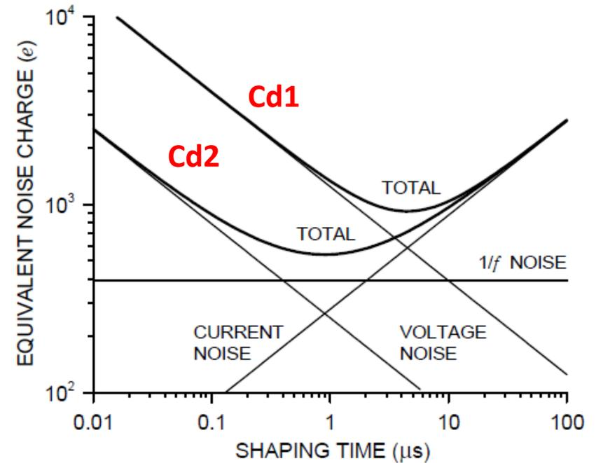
ENC using a simple CR-RC shaper with peaking time  $T$ :
