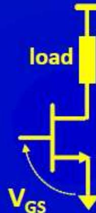
$V_{GS} \ll V_{th}$  (weak inversion)
