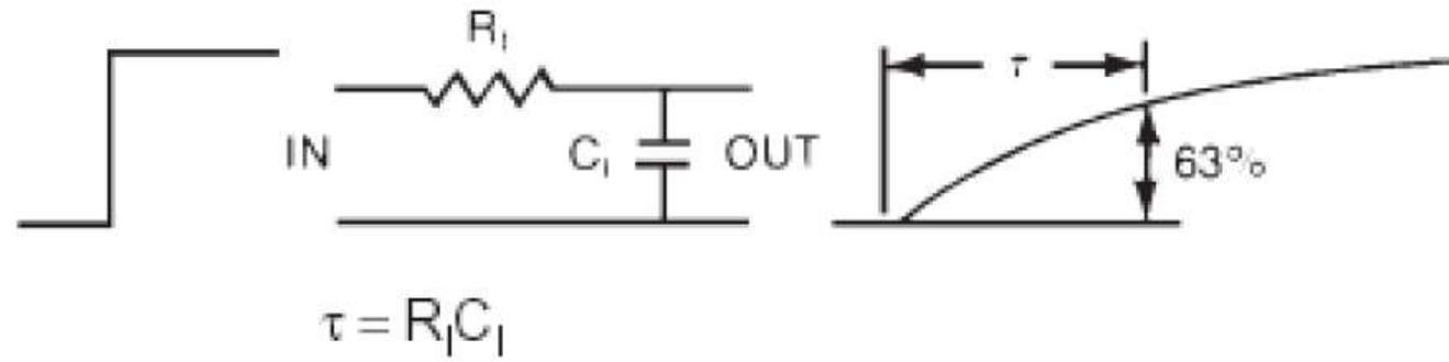
$$V_{in}(t) = i(t)R + V_{out}(t) \quad \text{and} \quad i(t) = \frac{dQ(t)}{dt} = C \frac{dV_{out}(t)}{dt}$$
