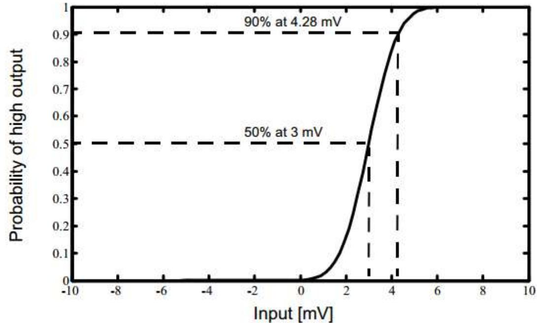
Probability of a high output logic level with varying input level for a particular comparator
