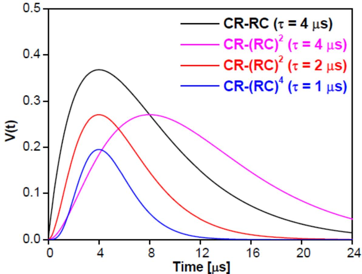
If a single CR high-pass filter is followed by several stages of RC integration, the output pulse shape becomes close to Gaussian amplifiers shaping, in this way are called **semi-Gaussian shaper**. Its output pulse is given by:
