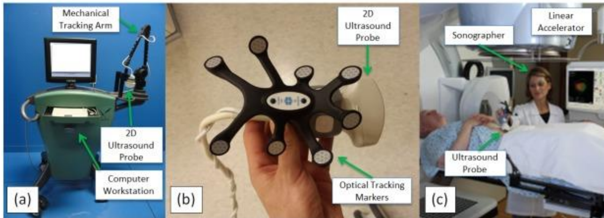
(a) NOMOS B-mode Acquisition and Targeting (BAT), courtesy of Medicka Medical LLC. (b) Elekta Clarity probe. (c) Clarity. From Western et al 2015
