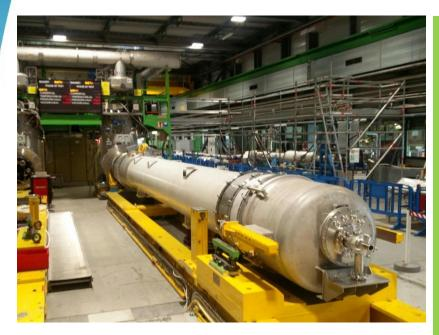
Inner triplet prototype MXQFB (coil length: 7.2 m) was tested @ SM18
