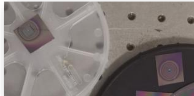
2 Fresnel Zone Plates of size ~23 mm x 23 mm
