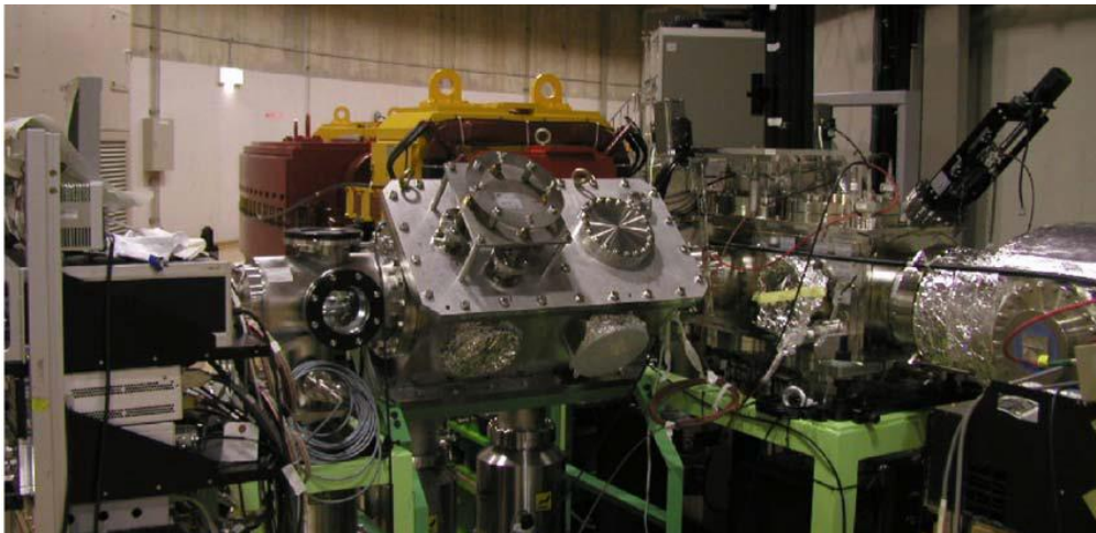
Gas jet monitor installed in the HIMAC synchrotron
