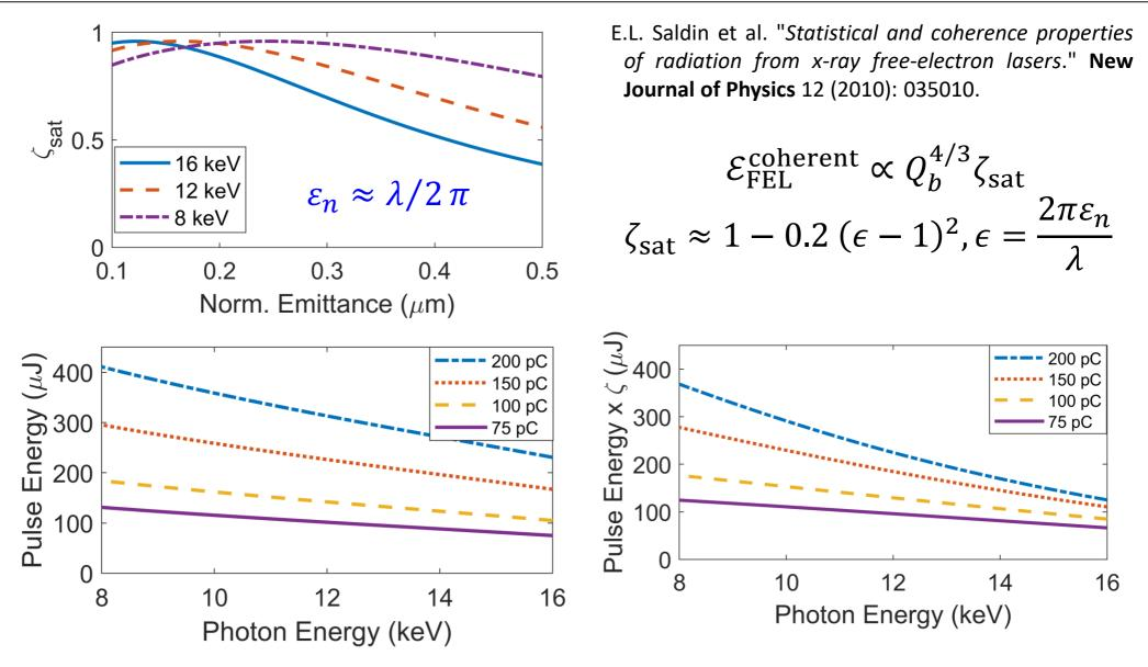
The **emitted coherent pulse energy doubles for 150 pC bunches** despite emittance degradation and some decline in the degree of transverse coherence.
