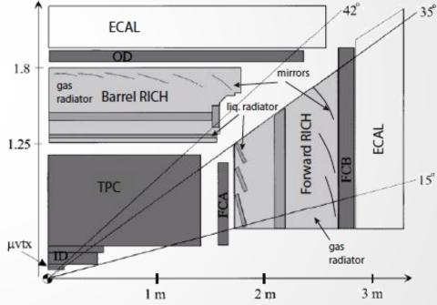
2. (bottom) a liquid or solid thin radiator produces a ring originating from a single vertex (no focusing mirror needed), e.g.  $\pi/K/p$  discrimination
