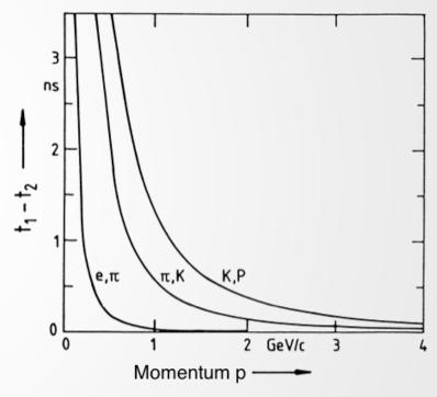
e.g.: Separate  $\pi$  from K with 4 standard deviations,  $\sigma_t = 0.3$  ns ( $\Delta t = 4 \sigma_t = 1.2$  ns)  $\rightarrow$  L  $\sim$  3 m at p = 1 GeV/c but already L  $\sim$ 12 m at p = 2 GeV/c
