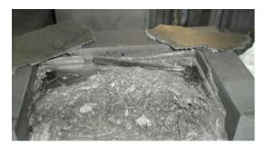
First test with 20vol.% pitch exploded the mould! It happened at ~400°C (decomposition temperature)
