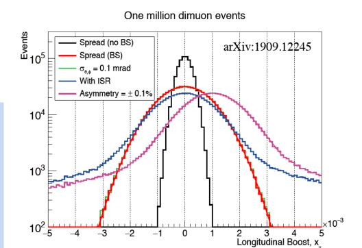
The measurement of CM boost distribution allows control of beam energy spread as well as the difference between e+ vs. e- energies.
