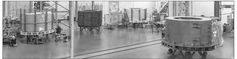
Four ITER CS production modules in various stages of fabrication
