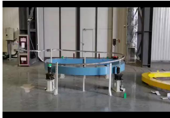
Verify the feasibility of sub-coil assembly and coil hoisting fixture design
