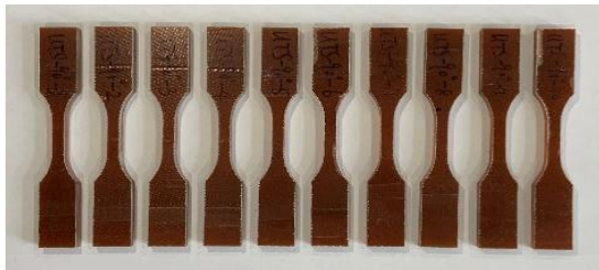
UTS (90/0 degree)_ASTM D 638
