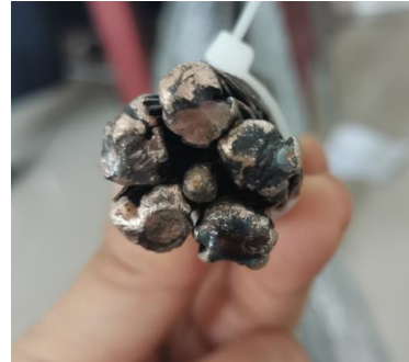
Sub-cable end welding
