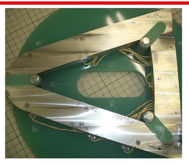
The damages of the coil look less from the appearance after electromagnetic force test.
