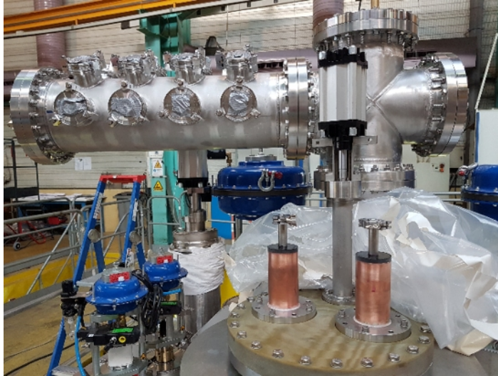
Top part of the cryogenic satellite with the warm extremities of the current leads, the cryogenic valves and one of the clarinets for the connectors interfacing 944 instrumentation wires for about 200 sensors.
