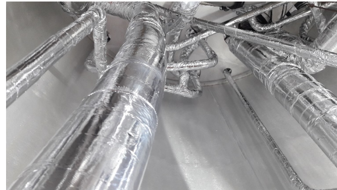
The cryogenic satellite of about 6 m high assembled at SDMS for pressure tests
