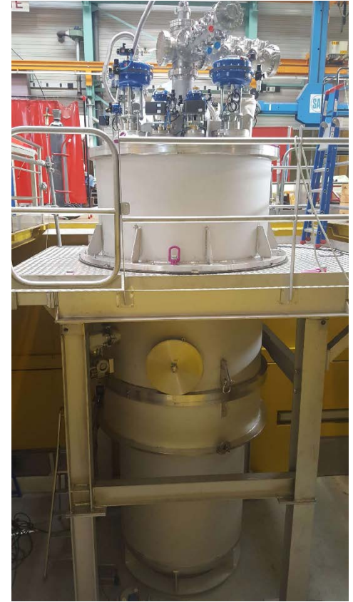
The cryogenic satellite of about 6 m high assembled at SDMS for pressure tests
