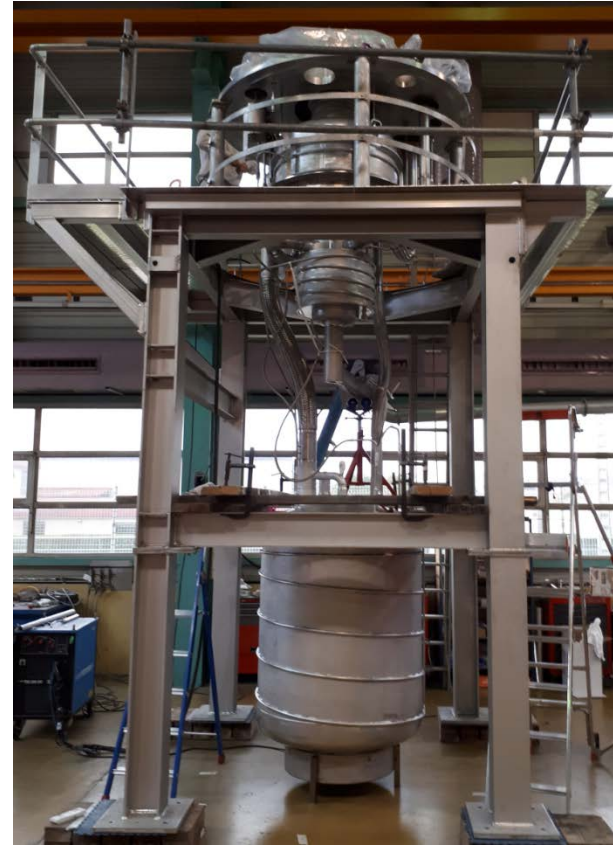
The cryogenic satellite of about 6 m high assembled at SDMS for pressure tests
