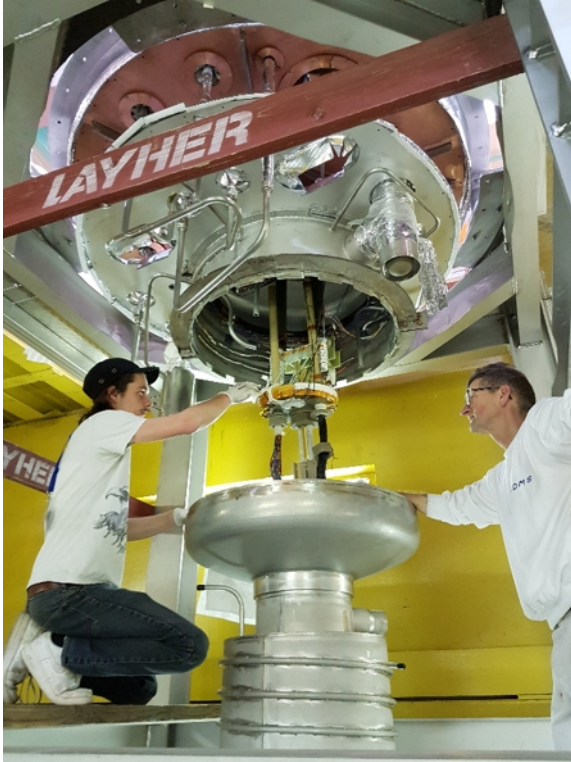
Mounting of the current leads and instrumentation wires crossing the \lambda -plate within the cryogenic satellite before the closure of the 4.2 K reservoir.
