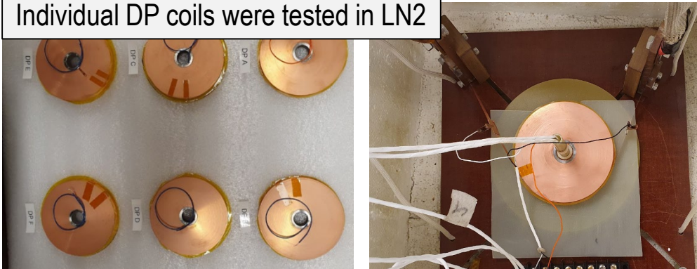
Extra shunting by soldering with 52In48Sn and completed DP coils
