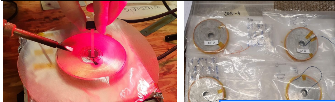
Extra shunting by soldering with 52In48Sn and completed DP coils
