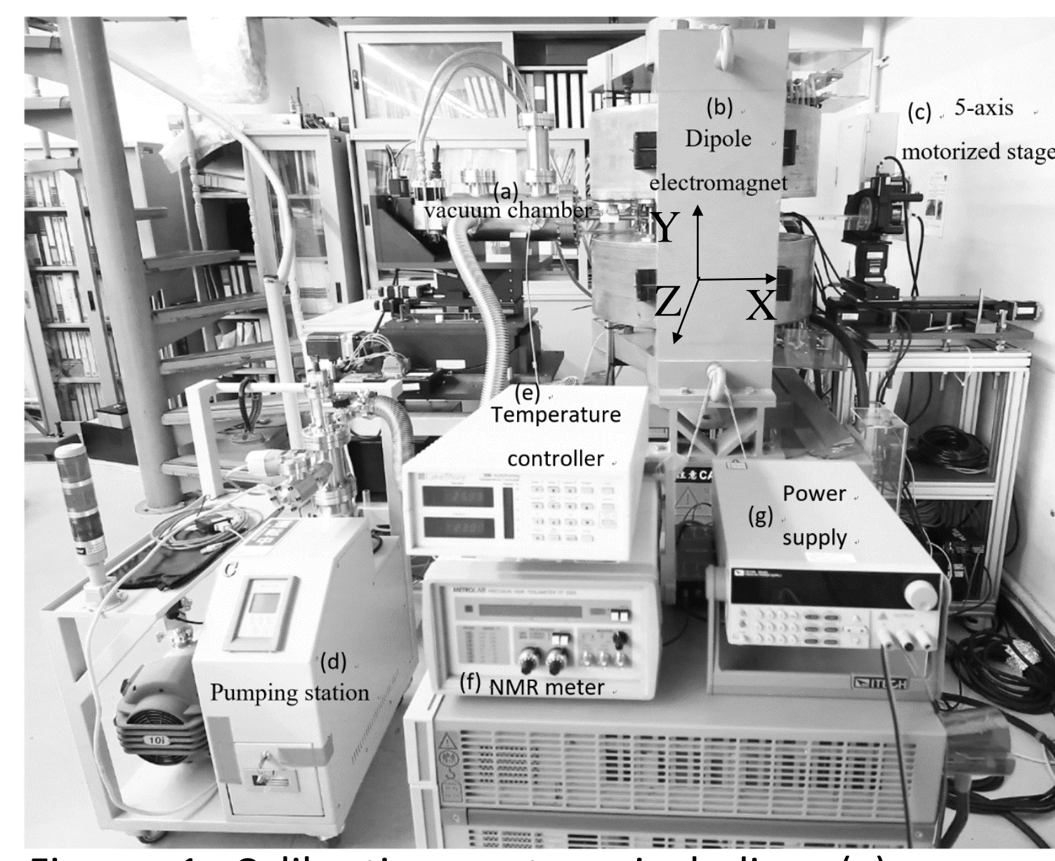
Figure 1 Calibration system including (a) vacuum chamber, (b) dipole electromagnet, (c) five-axis motorized stage, (d) pumping station, (e) temperature-control system, (f) NMR meter and (g) power supply
