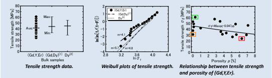
Tensile strength data of (Gd,Y,Er) are comparable to those of (Gd,Dy) and Dy. Weibull coefficient of (Gd,Y,Er) is slightly smaller than those of (Gd,Dy) and Dy. Tensile strength increases with decrease of porosity.
