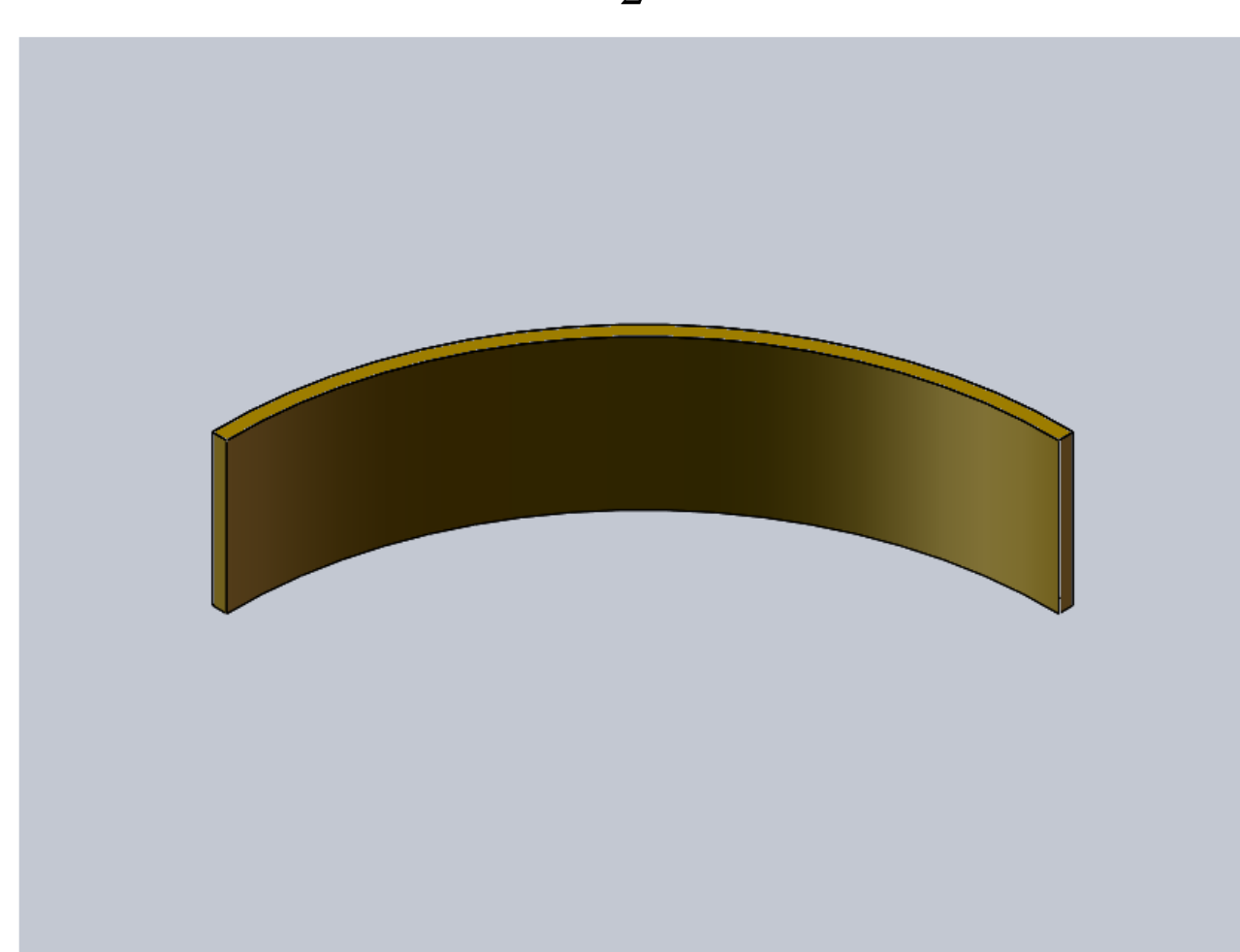
Fig. 3. Schematic view of REBCO tape under out-of-plane bending load.
