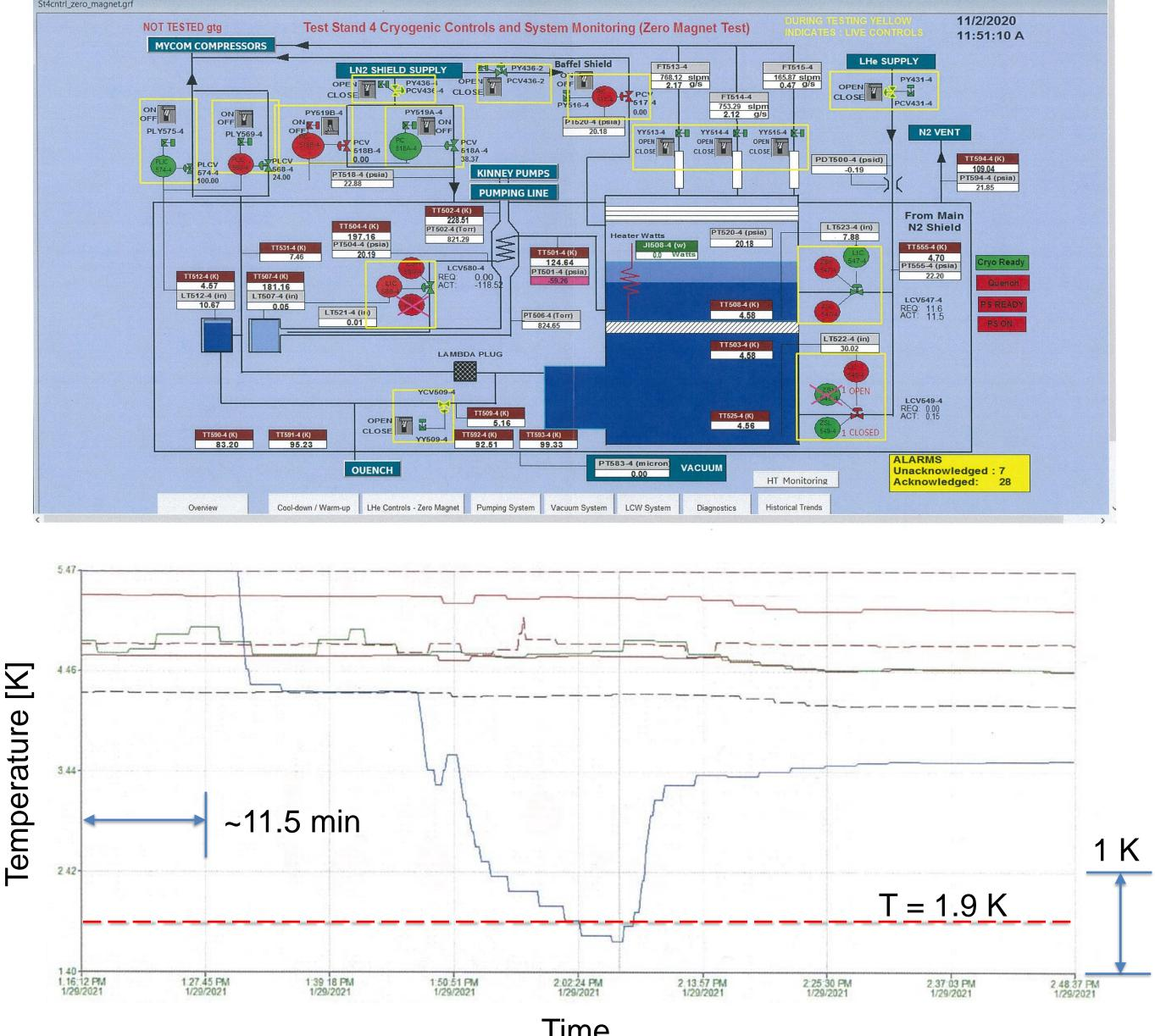
A Siemens 545 PLC was replaced with a Siemens S7 PLC for cryogenic process control. The original operator interface screens and historical data collection using Intellution Fix32 were upgraded to GE Digital iFix. A test stand monitoring screen and a historical plot showing cooldown of the upgraded pumping line to 1.9 K (blue line) are shown above.
