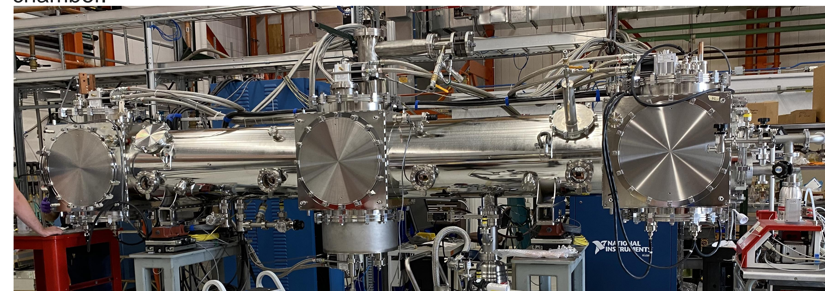
The thermal shield is cooled by all cryocooler 1 st stages
