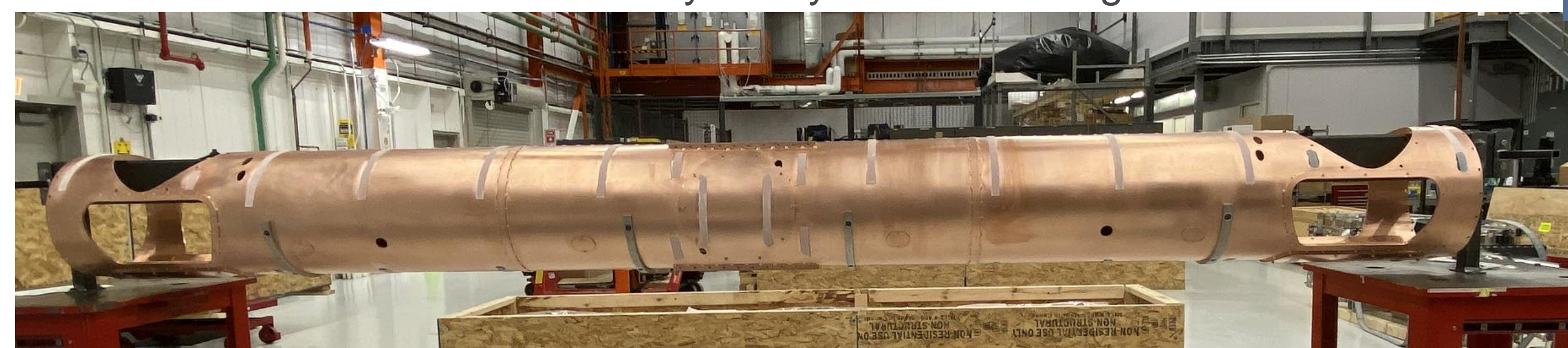
The thermal shield is cooled by all cryocooler 1 st stages
