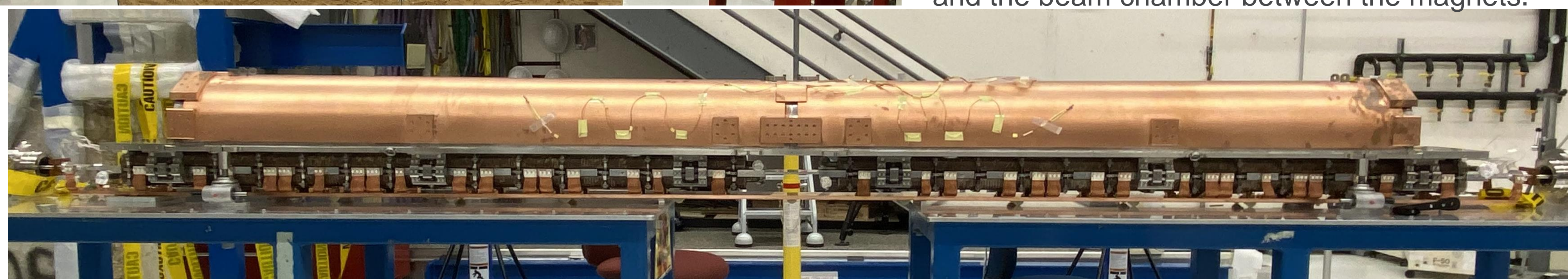
The cold mass: The cold mass consist of the two 1.9m superconducting undulators (four magnets) and the beam chamber between the magnets.
