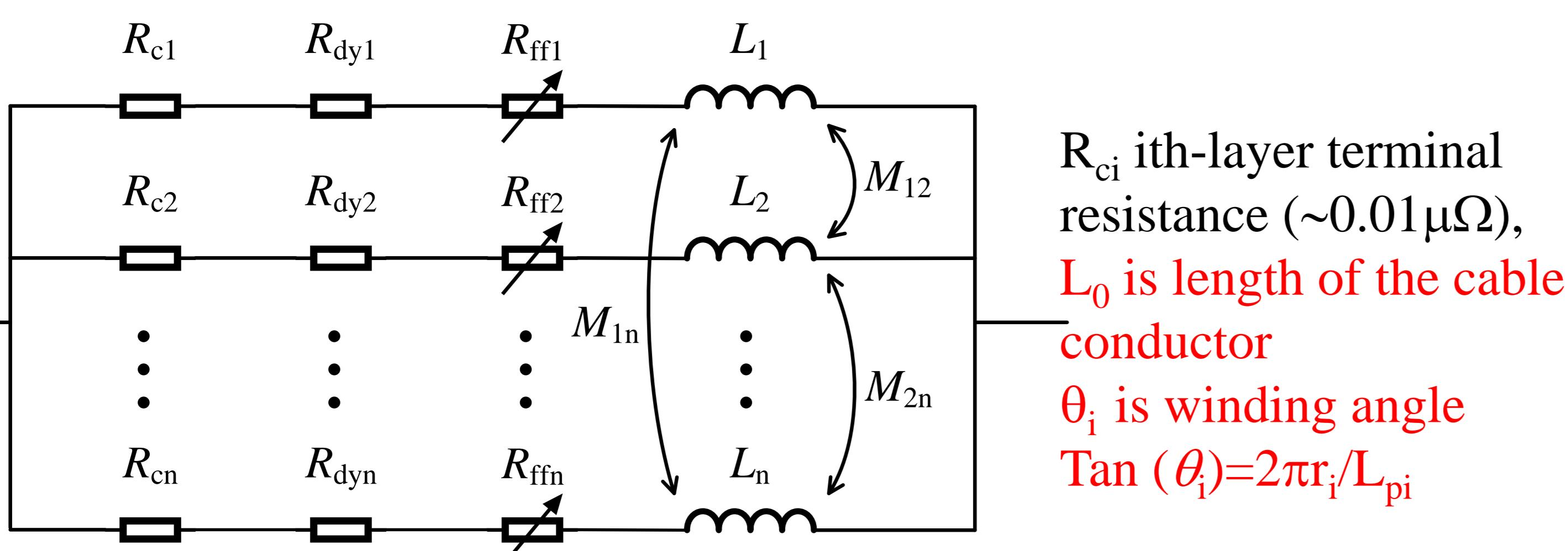
$R_{ci}$  ith-layer terminal resistance ( $\sim 0.01 \mu\Omega$ ),
