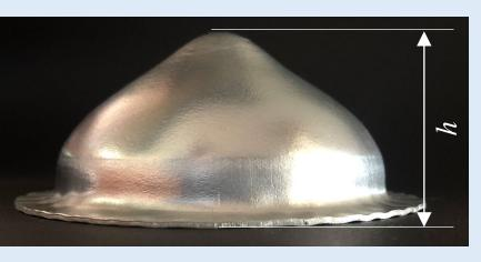
Figure 2 – Variable *h* (workpiece height).
