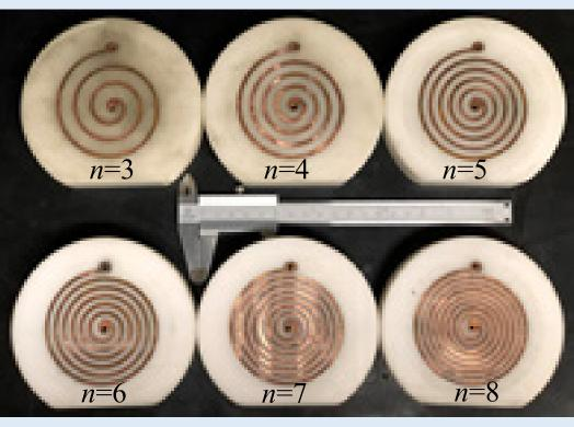
Figure 1 – Spiral coils used for parametric experiments.
