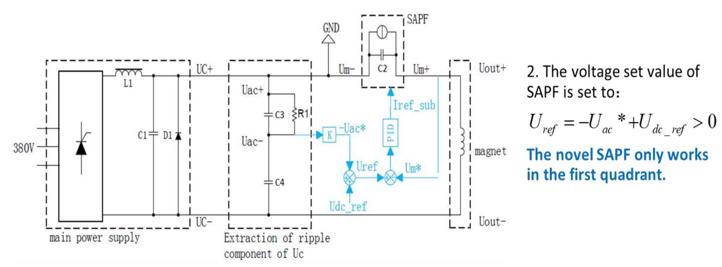
1. The novel SAPF is designed as a voltage source that directly tracks the negative value of the output voltage ripple of the main power supply (  $-U_{ac}*$  ).
