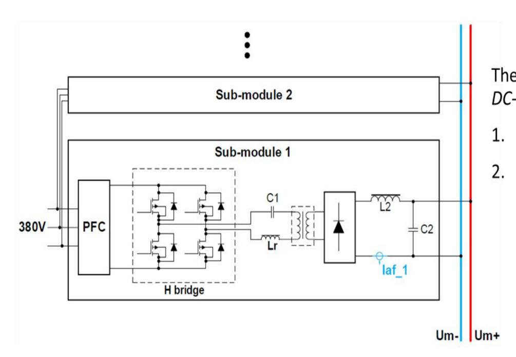
The novel SAPF is a conventional AC-*DC-DC* switching power supply:
