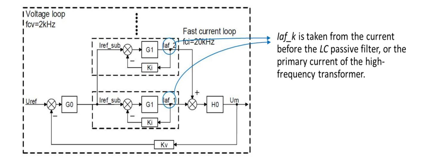
• 1. Fast current inner loop is used to realize automatic current equalization between sub-modules.
