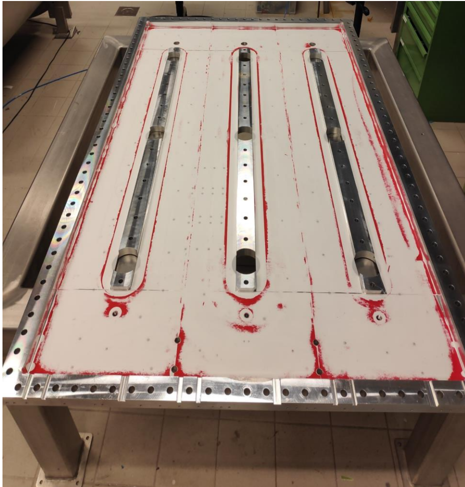
Fuji paper – Good contact around bolts
