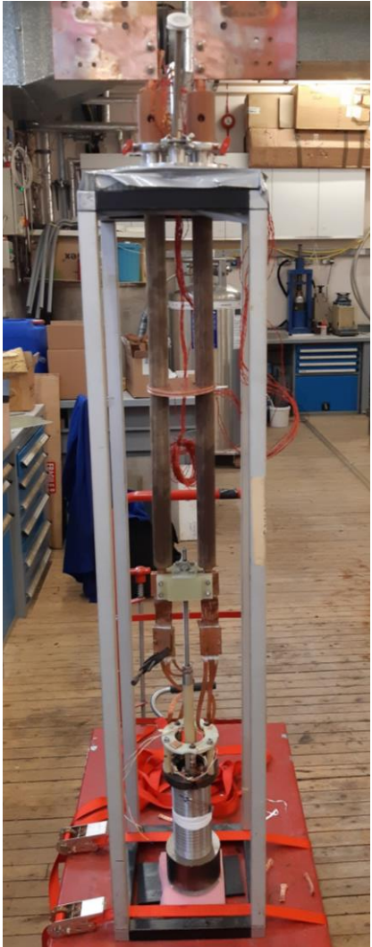
Left: coil set up for test rig
