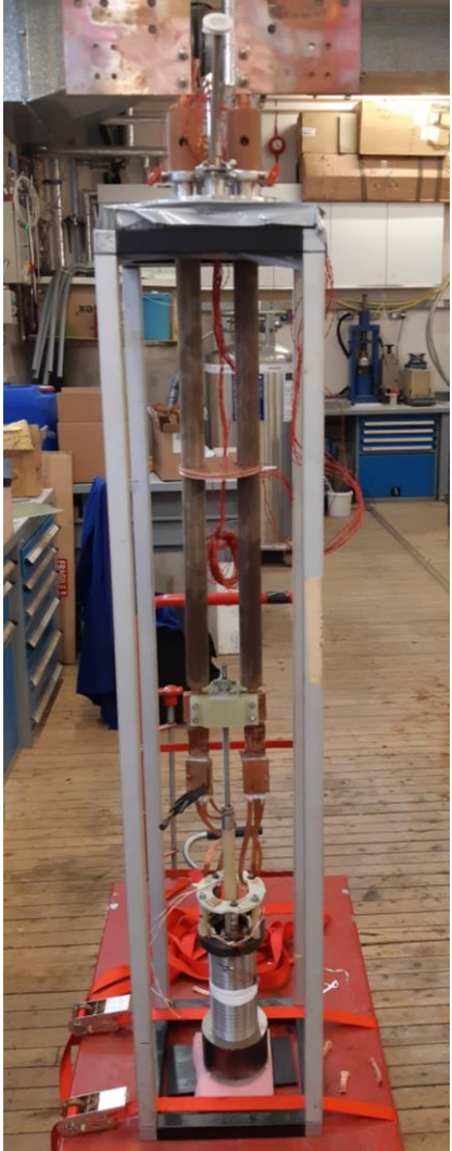
Left: coil set up for test rig
